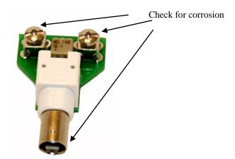
Check antenna loop for proper resistance. Disconnect the antenna loop from the balun terminals and measure between the two ends of the loop. It should read about 470 ohms. If it is within  $\pm$ 0 ohms then the reading is ok. If you see large resistance or an open it means there is a break in the loop.
