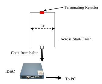
Generally the longer the loop is, the less detection height you'll get. The latest generation equipment has a great deal of sensitivity. Thus it is possible to stretch the loop out and still have enough detection distance. Some testing should be done before the loop is completely buried to verify that adequate performance exists.
