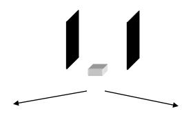
**Good location**: No metal to block the signal. The detection window is very wide.
