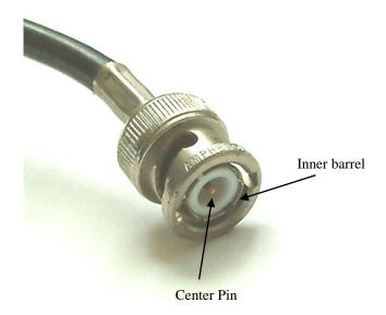
Make sure the center pin and inner barrel are flush on both ends of the cable. This is often the source of low hit numbers.
